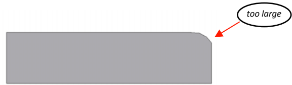
Guide bearing too large (radius incomplete)
