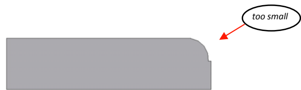
Guide bearing too small (radius cuts into material)
