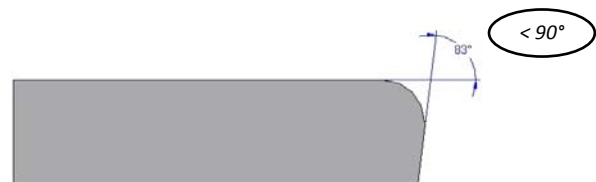
Angle less than 90° (radius cuts into material)
